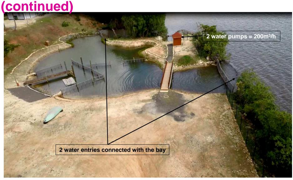
Renewal by the pumps of the volume of water in 10h besides the external supply made possible by the two openings on the bay
